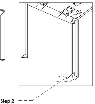
**Note:** Cable Channels magnetically attach to legs.
