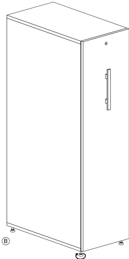
Ⓑ Slide the cabinet in place and level using adjustable glides
