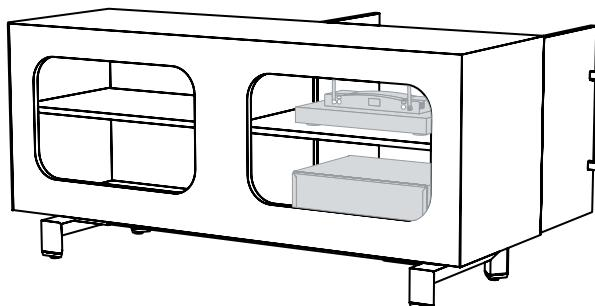
**Note** — The open back allows for appropriate technology ventilation and easy access for cable and technology installation.
